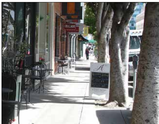
Sidewalk sign located to maintain accessible route.
