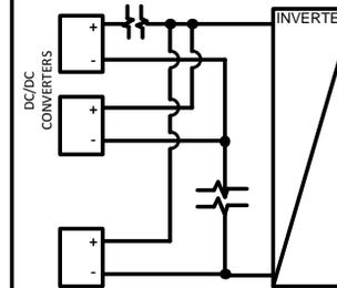
PARALLEL DC/DC CONVERTERS ON ONE SOURCE CIRCUIT (FIXED UNIT VOLTAGE DC/DC CONVERTERS)
